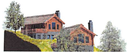
Construction on steep slopes should attempt to avoid excessive cutting into existing topography for foundations.
